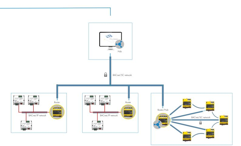
A possible BACnet/SC scenario: A head office for building management with SAUTER Vision Center as BACnet/SC hub, several properties with BACnet/IP and a BACnet/SC extension in the network.
